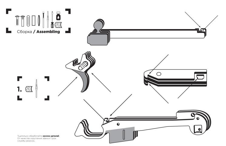
Carefully file down **the sides**. Elastic band lifetime depends on how carefully you have filed the burrs!
